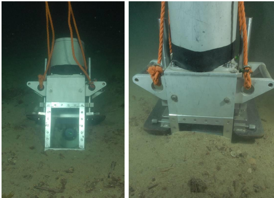
Figure 7.1. Diver operated Sediment Profile Imaging camera. The left-hand image gives a view of the camera at the sediment surface. The right-hand image shows the SPI camera when inserted into the sediment.
